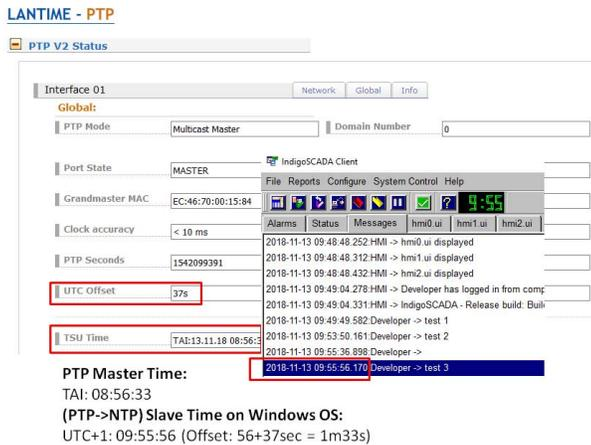
**Figure 3** Snapshot of PTP synchronized timestamping done at Windows OS
