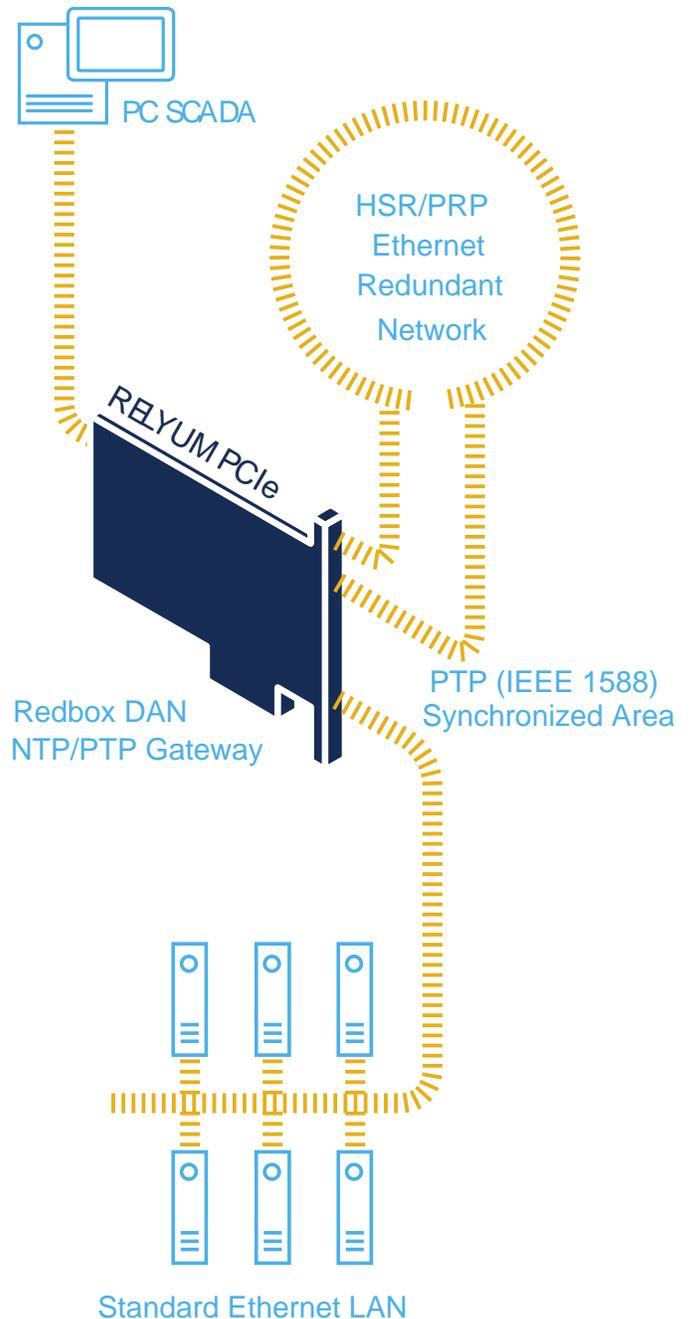
**Figure 1** Merging PTP Networks (legacy and high availability) with NTP synchronized systems.
